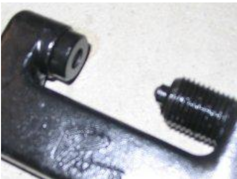
We now configure the tool as a fixed press with an anvil to hold the head of the rivet, and a heavy riveting pin to spread the open end of the rivet.
