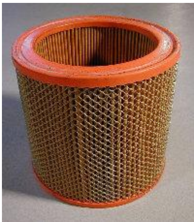
The stock disposable element. Paper pleats with a wide wire mesh on the exit side of the element.
