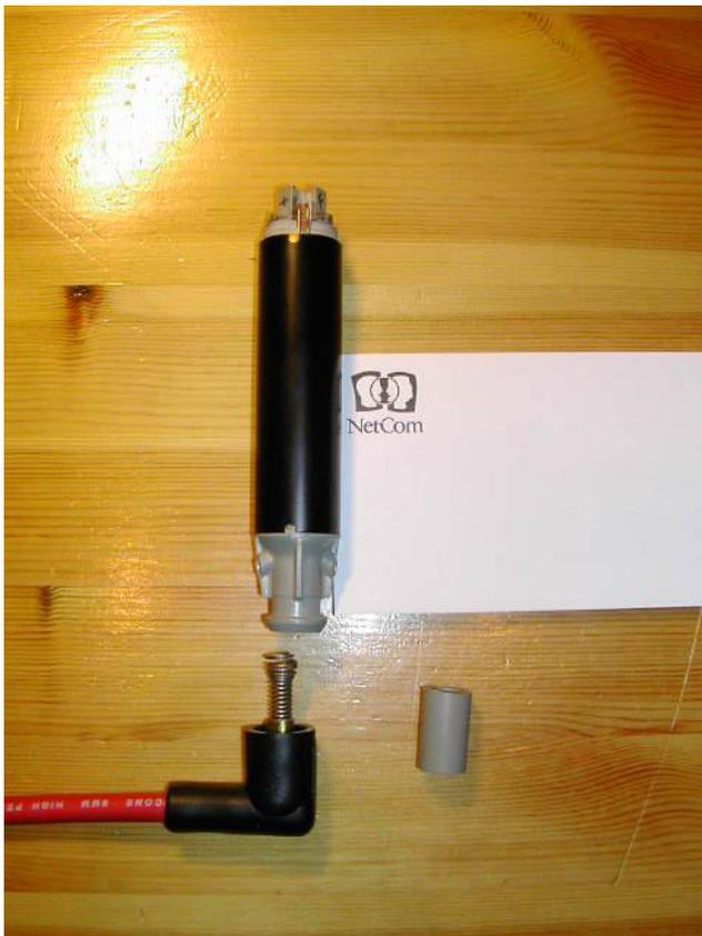
Where did you buy the plug wires? I used the OEM ones still, and since they come out straight there is very little room for mounting since the new coils are longer. Looking at your pictures, how did you attach the plug wire to the coil? For me, the rubber boot did not provide a real secure connection (would slide right off). I just pushed it in and taped the heck out of it. Ugly but effective.
